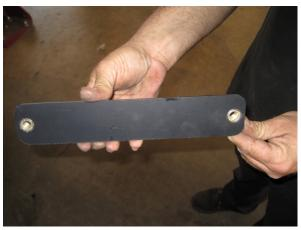
This flat bracket uses two 3/8" dia nut-serts as shown.
