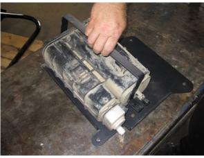
Place cannister on the new PJ skid plate and align bracket with bolt holes.
