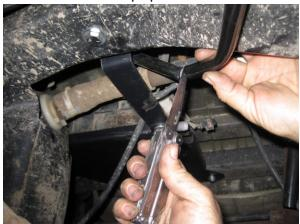
Cut factory hose just after the bend as shown. Save the cut end to be re-used.
