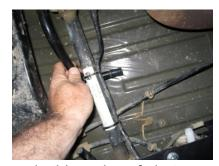
Rotate and route the factory hose over the cross-brace as shown in this series of photos.
