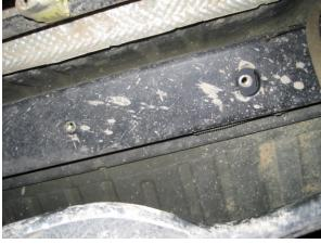
Align Nut-serts with holes in cross-brace. Reinstall the body mount bolt on 4-Door.
