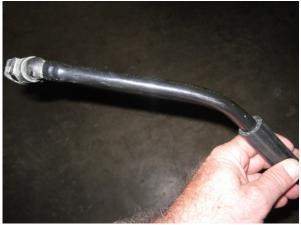
Mount new rubber hose to the cut end of the factory hose.
