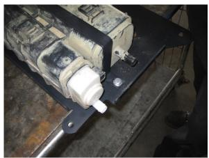
Bolt the two pieces together using the 3/8x 1" bolts, nuts, and flat washers.
