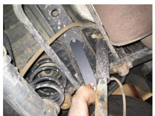
Insert the flat bracket into the frame channel as shown. Make sure the nut-serts are in the "Face-Up" position.
