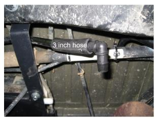
Insert plastic elbow into cut factory tube.
